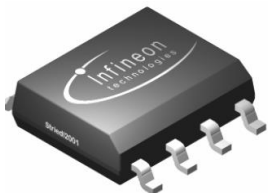
Giant Magneto Resistance (GMR) sensor
